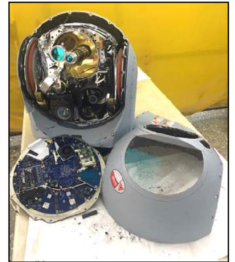
Bayraktar TB2 imaging and targeting system manufactured by a Canadian company
